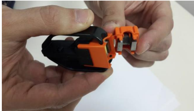
Figure 5. Press the opener to release the cover.
